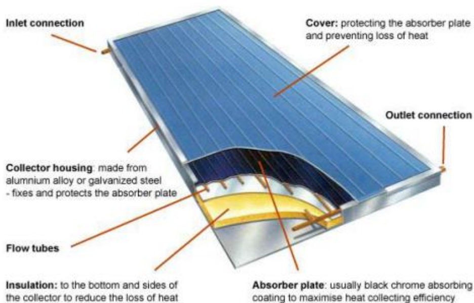
Figure 2.6: Typical Flat-plate solar collector
