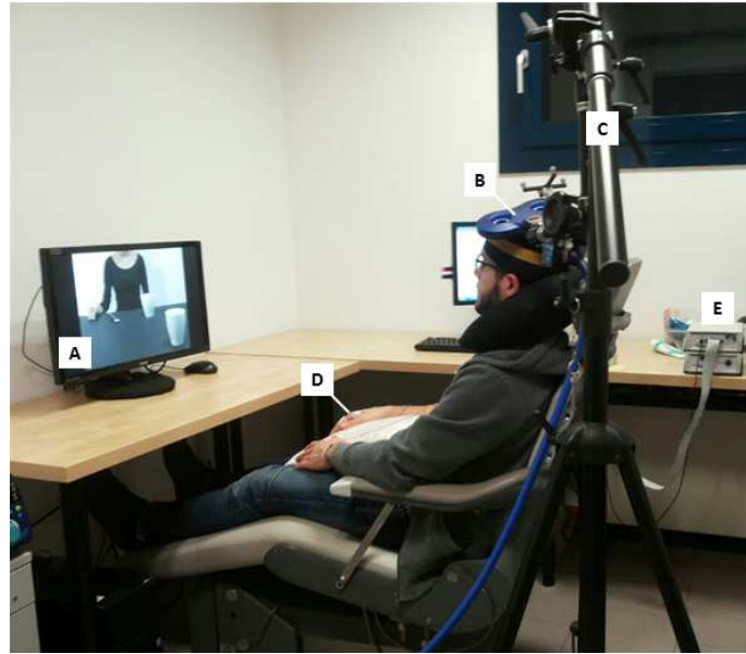
Figure 4.2: The laboratory set-up for TMS experiments, showing: A) the screen from which the experimental videos were presented; B) the TMS figure-of-eight coil; C) the TMS coil holder tripod; D) the EMG electrodes; E) the EMG amplifier.
