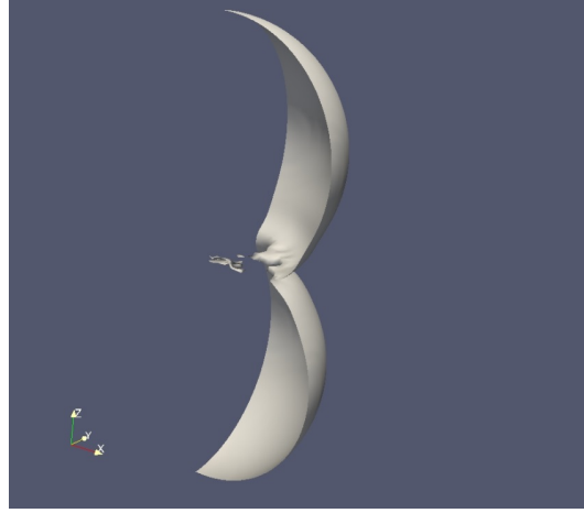
Figure 3.3.: Unphysical interface oscillation near contact area in a binary droplet collision. Three symmetry planes are employed in the simulation.
