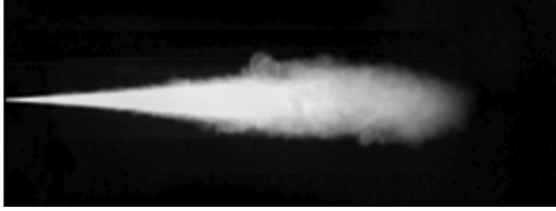
Figure 1.2.: Diesel spray imaged by Wang et al. [67]
