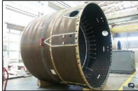
Anisogrid composite lattice structures - Development and aerospace applications; V.V. Vasilev, I. VA. Barinov, A.F. Razin
