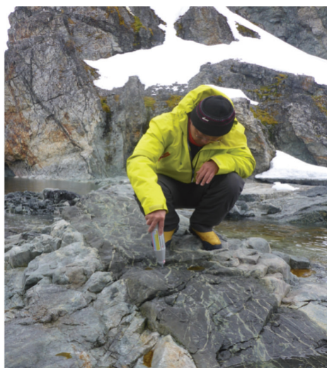
FIGURE 2. Schmidt hammer rebound test at Graham Coast, Antarctic Peninsula
