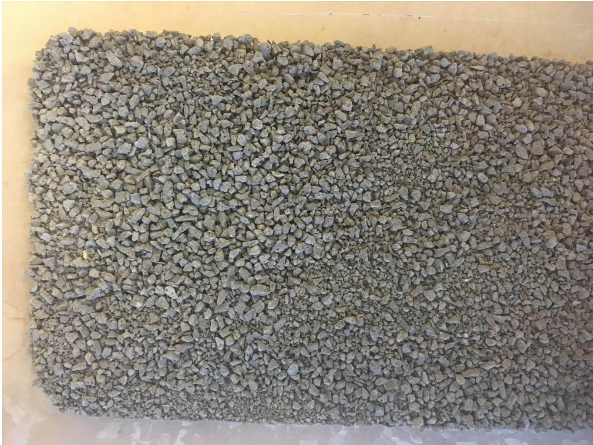
Figure 2.1: Clay granules made with peat containing B. spp. and crushed to the market size of between 0.5-2.5mm.
