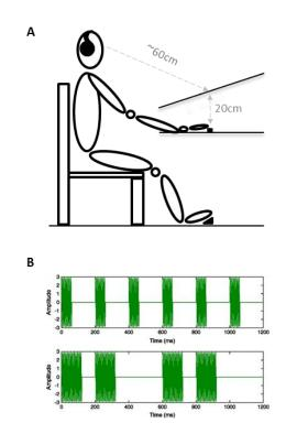
**Figure 12 Experimental setup and features of tactile targets.** (A) Graphic illustration of experimental set up. (B) Waveforms of two tactile targets. The upper panel indicates the waveform of Target 1 (T1), a 5-Hz square wave with a 30 % duty cycle delivered via 150-Hz vibrations. The lower panel shows the waveform of Target 2 (T2), a burst square wave (mean frequency of 4.17 Hz) with an average 30 % duty cycle delivered via 150-Hz vibrations.
