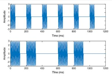
Fig. 5 Waveforms of two tactile targets. The upper panel indicates the waveform of Target 1 (T1), a 5-Hz square wave with a 30 % duty cycle delivered via 150-Hz vibrations. The lower panel shows the waveform of
