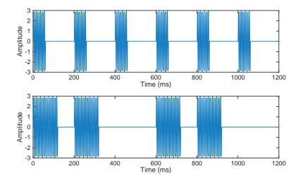
**Figure 7** Waveforms of two tactile targets. The upper panel indicates the waveform of Target 1 (T1), a 5-Hz square wave with 30% duty cycle delivered via 150-Hz vibrations. The lower panel shows the waveform of Target 2 (T2), a burst square wave (mean frequency of 4.17 Hz) with an average 30% duty cycle delivered via 150 Hz-vibrations. The distractors are constant vibrations of 150 Hz.
