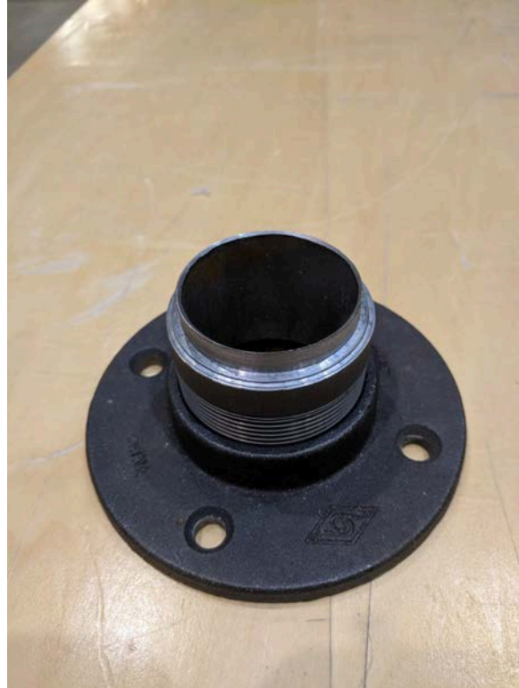
Figure 10. Show is the facing of the steel pipe and the finished punch
