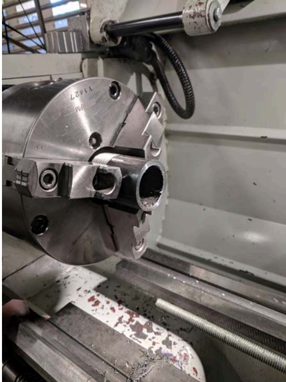
Figure 10. Show is the facing of the steel pipe and the finished punch
