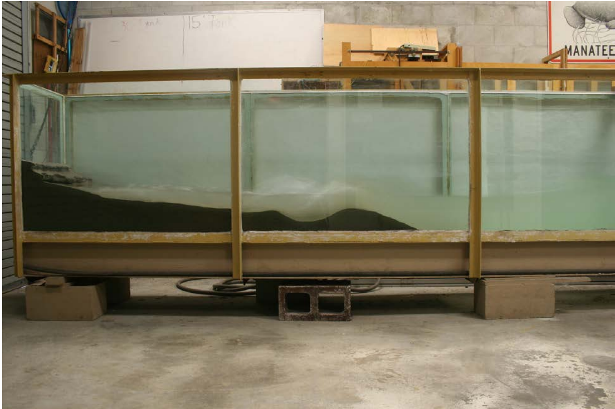
Figure 11: Example of a coastline used in Florida Institute of Technology's wave tank
