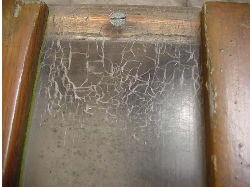
Figure 26. How acrylic fractures
