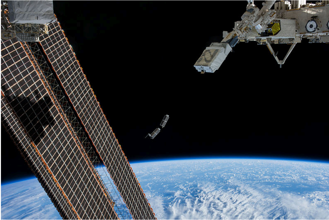
Figure 2. Daughter Nanosatellite Deployment [3]
