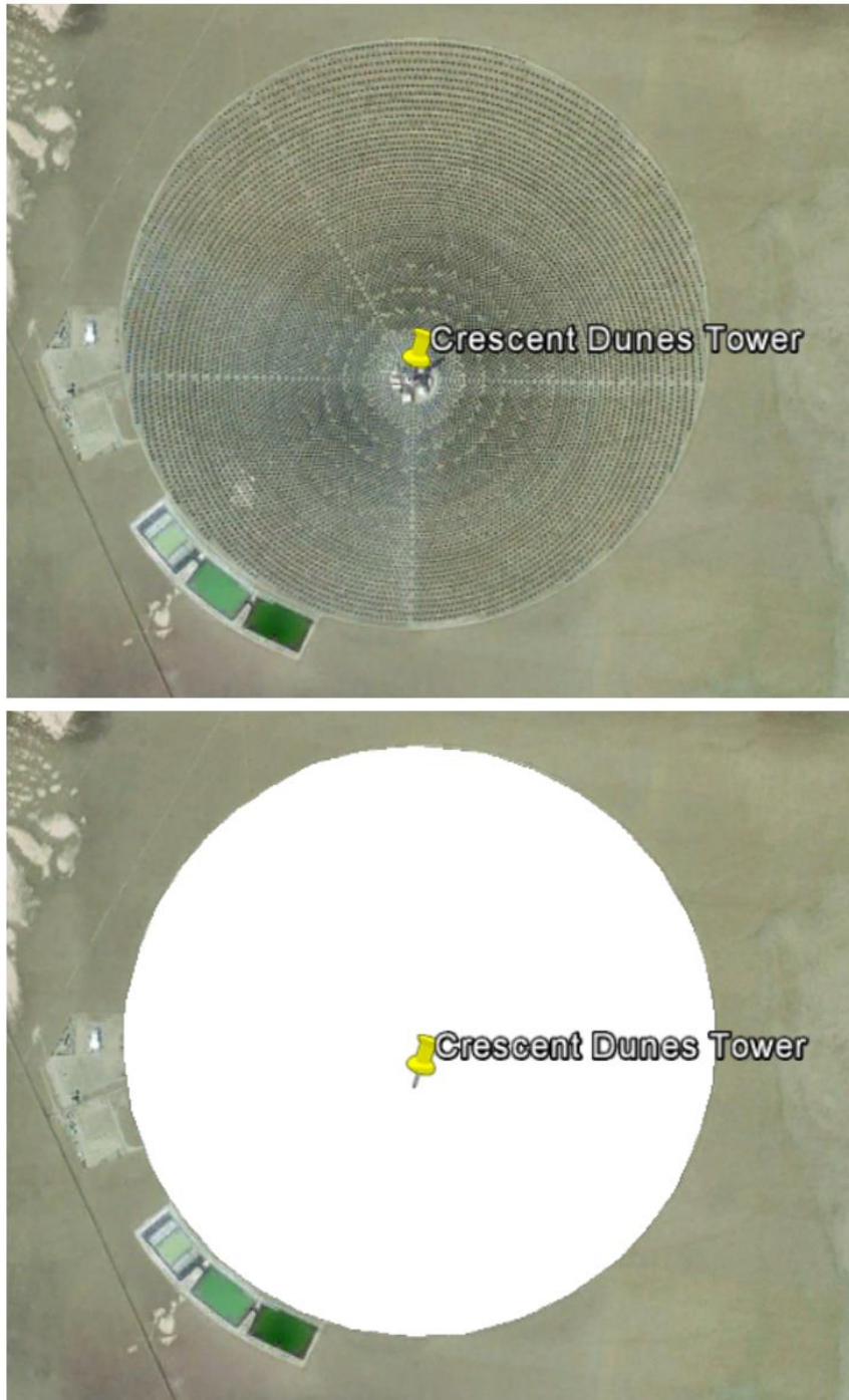
Figure 4-17: SolarPILOT validation, layout setup - field land boundary array of the actual project (picture originally from Google earth PRO)
