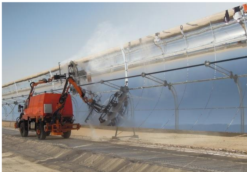
Figure 4-52: Truck with cleaning arm with brush [80]
