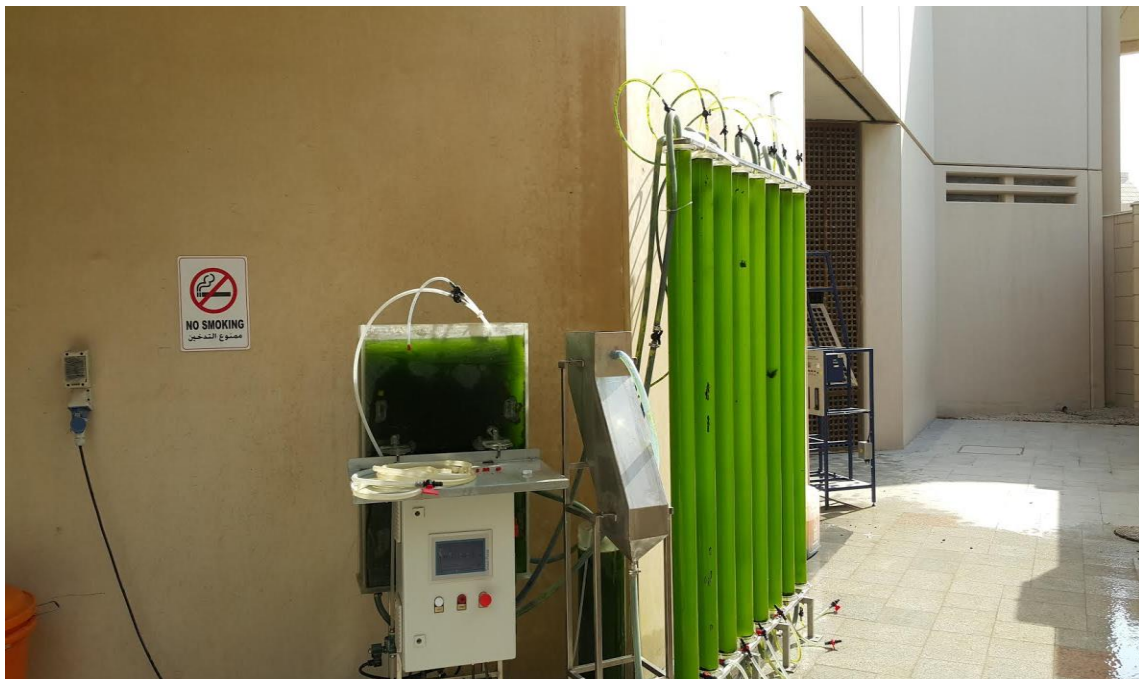
Figure 3.5: Pilot Plant PBR under operation
