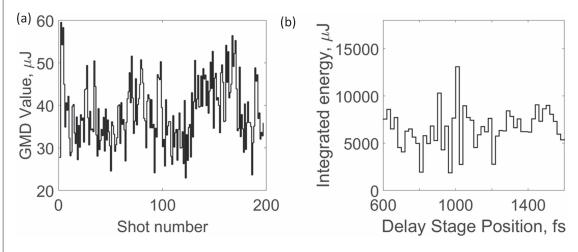
Figure 4. (a) Shot-to-shot XUV pulse energy as measured by the GMD for the first 200 shots of the delay scan. (b) Integrated XUV pulse energy for each delay stage position.
