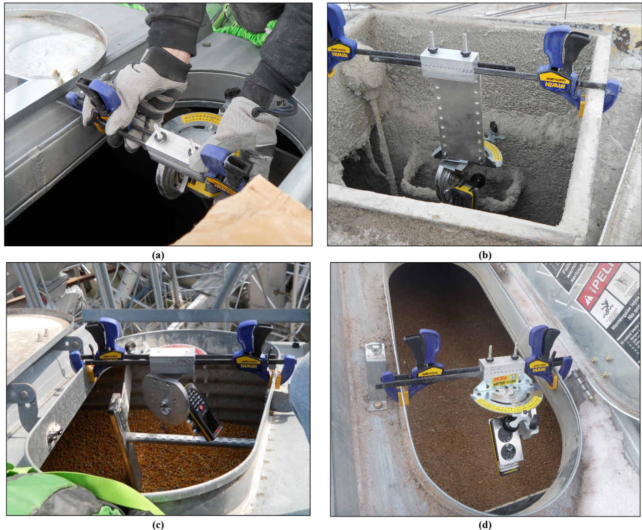
Figure 1. Bin measuring system being mounted on a typical steel bin (a), use on a concrete silo (b), and final mounting on two bins (c) and (d).
