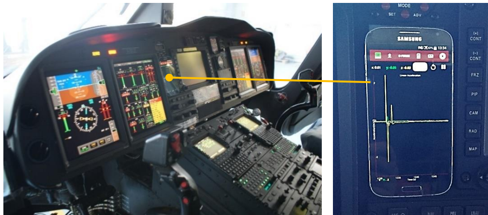
Figure 5.4 In-situ Vibration Measurement.
