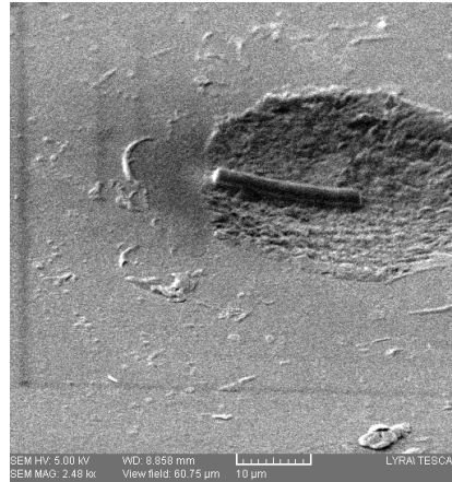
FIGURE 3.16 : SEM of a crater with Platinum deposited on the area used for the lamella.
