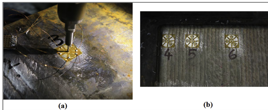
Fig. 13. Residual stress measurements made by incremental hole drilling in the buttering layer (a) and in the cladding overlay (b).
