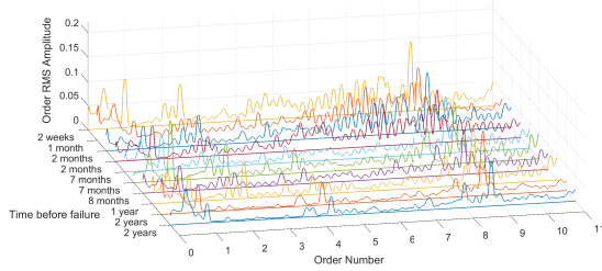
Figure 5. Order Spectra of Intermediate Speed Shaft Acceleration for Varying Times Prior to Failure
