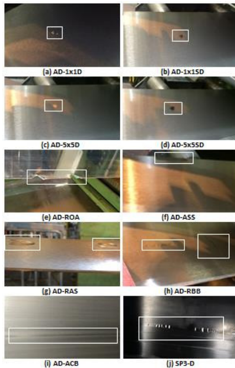
Figure 8. Defects in cold roll bonded Al/Al-Sn/Al/steel strips (a) 1x1 mm alumina, (b) 1x1 mm steel debris, (c) 5x5 mm alumina, (d) 5x5 mm steel debris, (e) run-off clad Al, (f) altered steel sanding, (g) rolled-in clad Al slivers, (h) rolled-in brush bristles, (i) altered clad Al brushing, (j) Al-1050 foil blisters on sacrificial side
