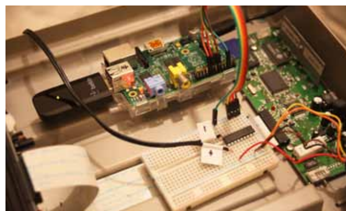
Fig. 3. Connection of the Raspberry Pi to the breadboard, and on to the flatbed scanner.
