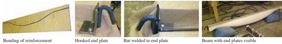
Figure 5 — Anchorage using welded end plates.
