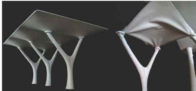
Figure 19 - Fabric cast columns supporting fabric formed shells (image courtesy CAST)
