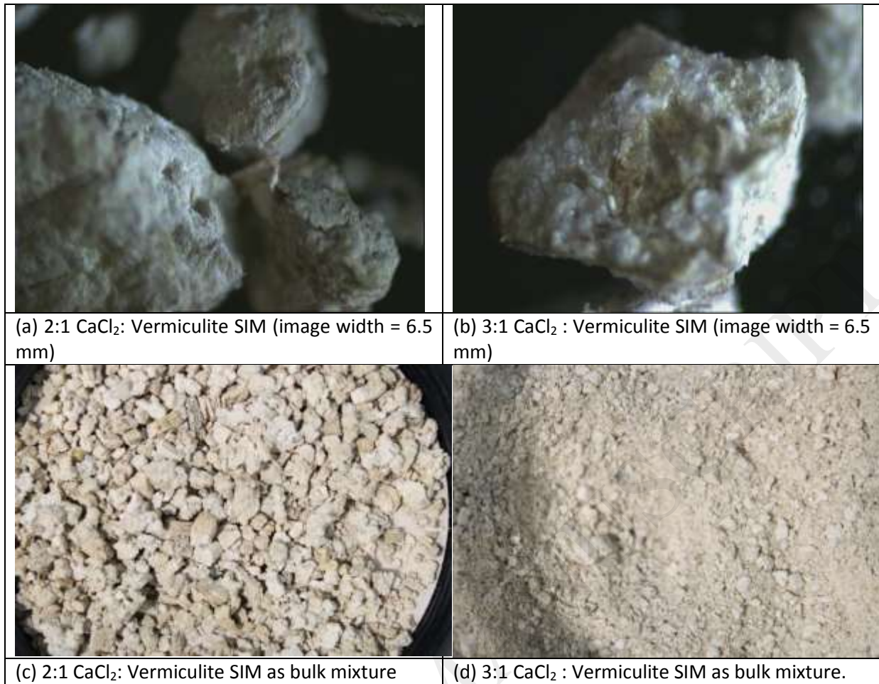
Figure 1 : Images of the CaCl 2 SIM material as prepared at (a) 2:1 Salt : vermiculite ratios used and (b) 3:1 salt : vermiculite ratio.
