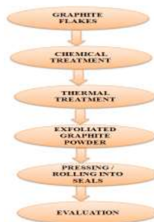
Fig. 1 – Process flow chart of exfoliated graphite product
