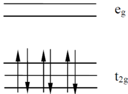
Fig. 2 – Electronic configuration for the low-spin case of the \text{Co}^{2+} ion in the octahedral environment of the \text{SnO}_2 rutile structure
