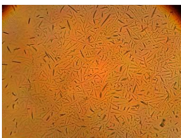
Fig. 4 – Micrograph of a film from a solution with a concentration of 25 g/l (magnification × 400)
