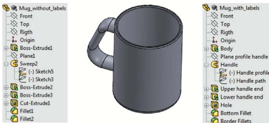
Figure 3. Proper labeling of modeling operations as a simple way to convey design intent. Default naming (right tree) vs. proper naming (left tree).
