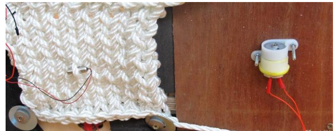
Figure 2: Vibromotors attached to back of button interface
