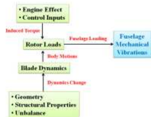
Fig. 4. Functional block diagram of helicopter vibrations.
