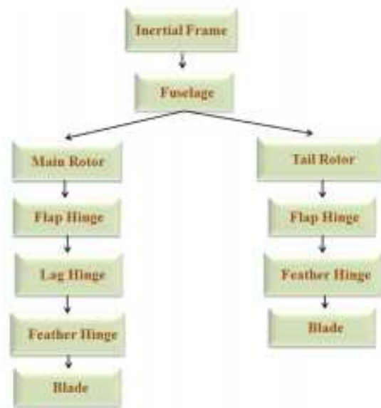
Fig. 6. Body structure diagram of the conventional model helicopter. Both main and tail rotor in this diagram contain one blade element only due to space restrictions, but the model can contain as many blades as needed.
