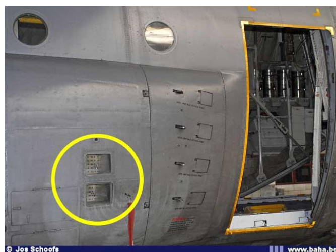
Figure 5-19 Position of flare dispensers in the aft end of the main landing gear fairings(87).
