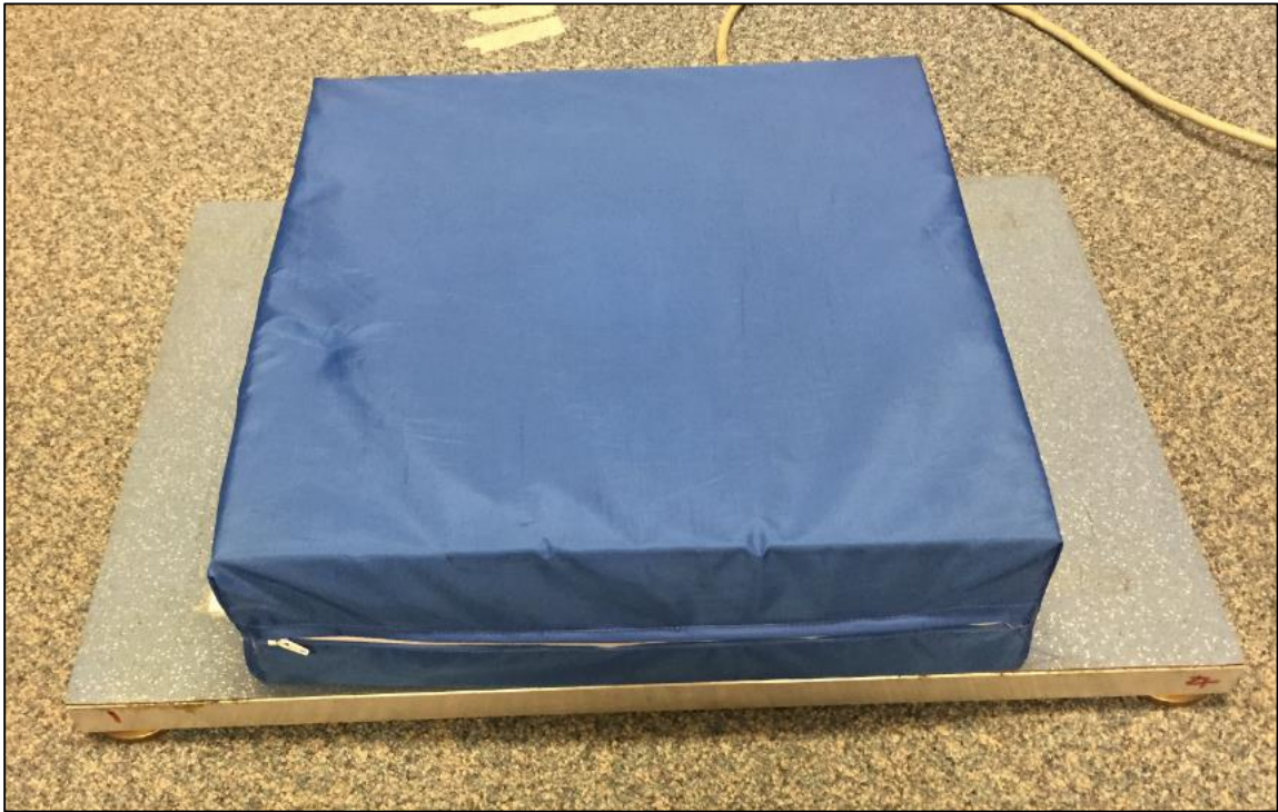
Figure 1 - A Foam (39 cm × 39 cm × 10 cm thickness) on a Force Plate
