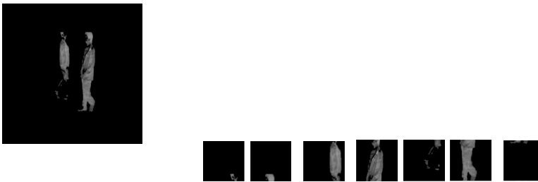
Fig. 4 the first image on the left is the background subtracted frame, the rest images are blocks containing the targets (with non-zero pixels)
