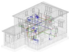
a) MEP layout (Autodesk Revit 2015)
