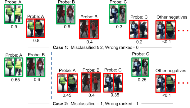
Figure 4. The binary classification loss prefers to training a lower misclassification rate model like Case 2 rather than Case 1, which imports a wrong order (Probe C). And it is an undesired locally optimal solution for person ReID. (Best viewed in color)
