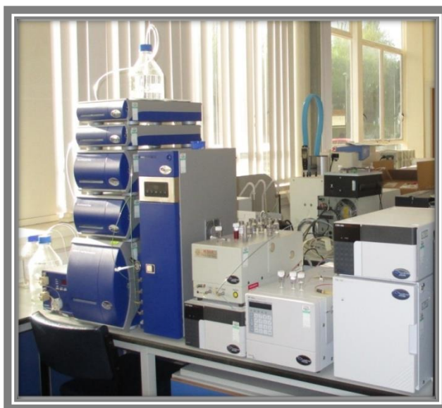
Figure 2-16 : Asymmetrical flow-field Flow fractionator (AF2000), Postnova Analytics.
