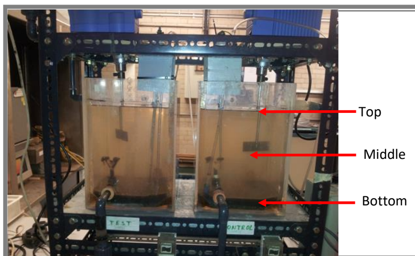
Figure 5-1: Sewage treatment in the SBR pilot WWTP after completion of the settlement phase.
