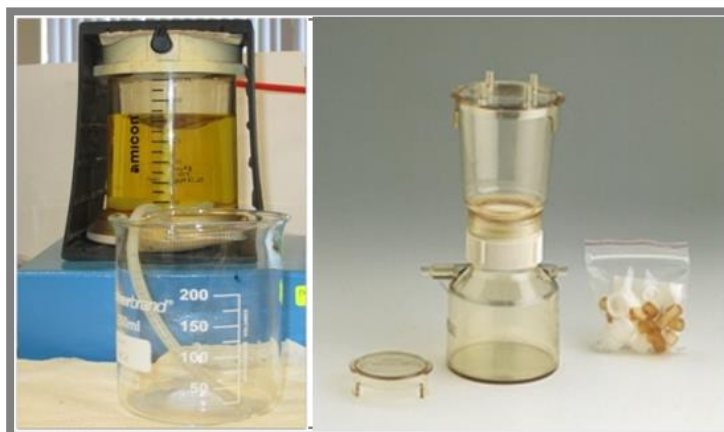
Figure 2-2: Millipore 400 mL ultrafiltration stirred cell (left image) and the 250 mL Millipore sterifil filter cell (right image, from (FisherScientific), UK)
