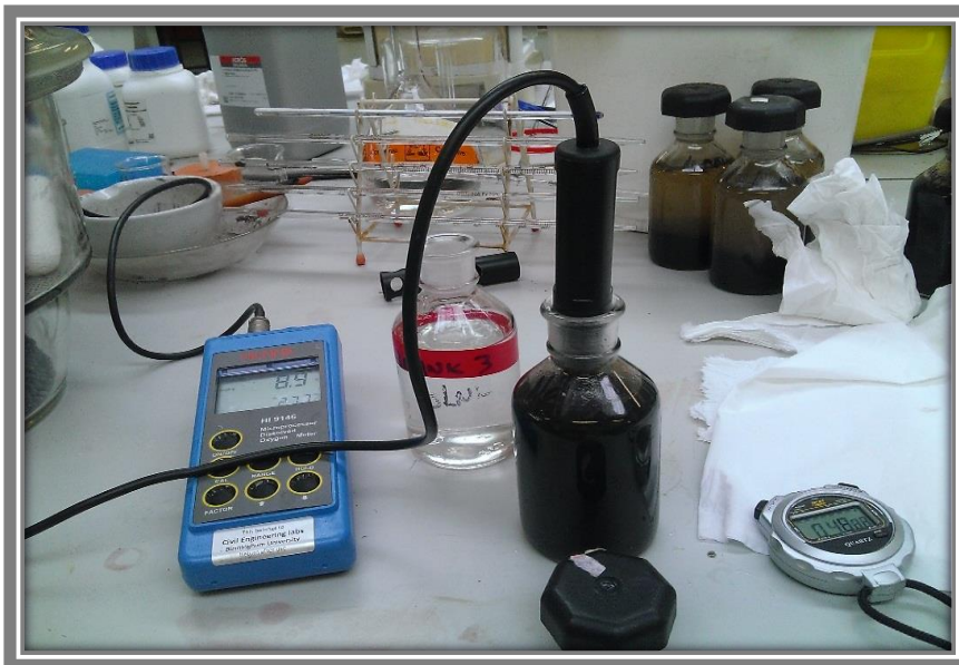
Figure 2-7: the 5-day biological oxygen demand measurement (using a microprocessor dissolved oxygen meter, HI 9146, Hanna instruments).
