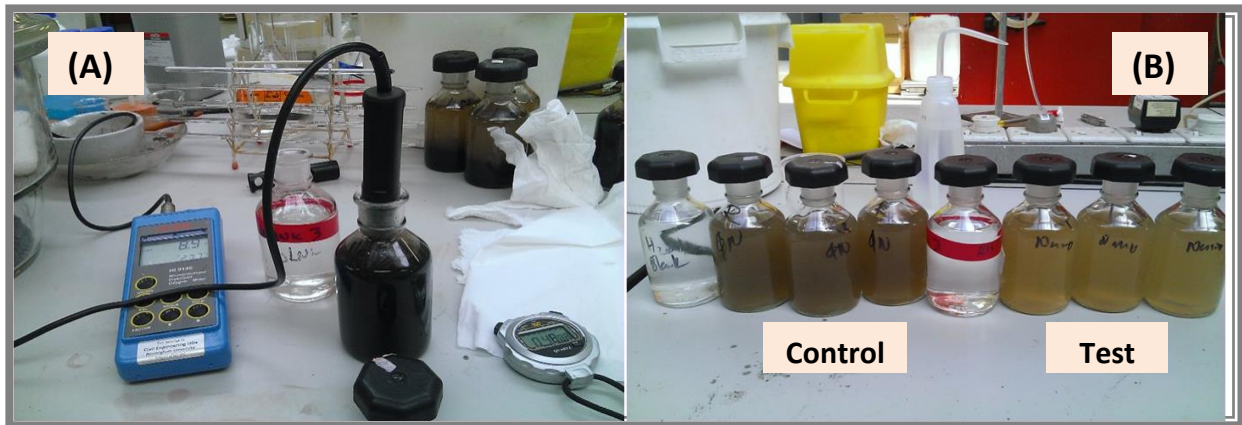
Figure 6-2: (A) - BOD 5 measurement experiment; (B) – test and control (without NPs or Ag + ) samples for BOD measurements in week 2 after incubation, test samples more clear than the control samples due the increase in settlement of the test sewage.
