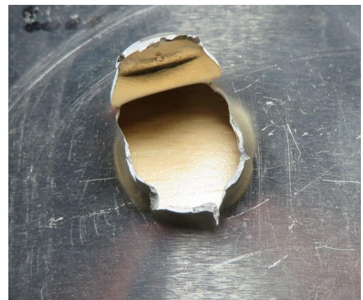
Figure 2.5 Transition in failure modes during impact perforation of thin AA 6082-T4 target with variation in projectile corner radius, numerical results based on MMC failure model (left) and experimental results (right), (a) R_c = 1.5 mm, (b) R_c = 3.0 mm, (c) R_c = 4.5 mm.
