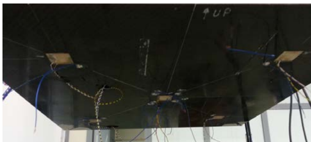
Fig. 10: Piezoceramic patches bonded on the panel
