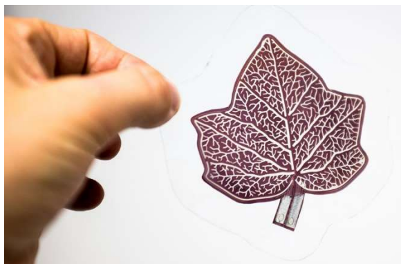
Figure 1.18 A flexible printed organic solar cell in a leaf motif. 79
