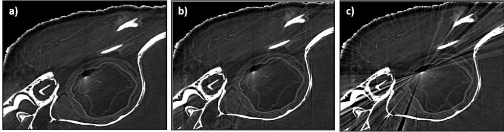
Figure 3.2: Reconstructed CT slices from unprocessed projections showing how image artefacts increase if the overlap position is not chosen accurately during the half-tomography correction. Resulting streaks due to shifting the overlap position by 0.5 (b) and 2.5 (c) pixels with respect to (a).
