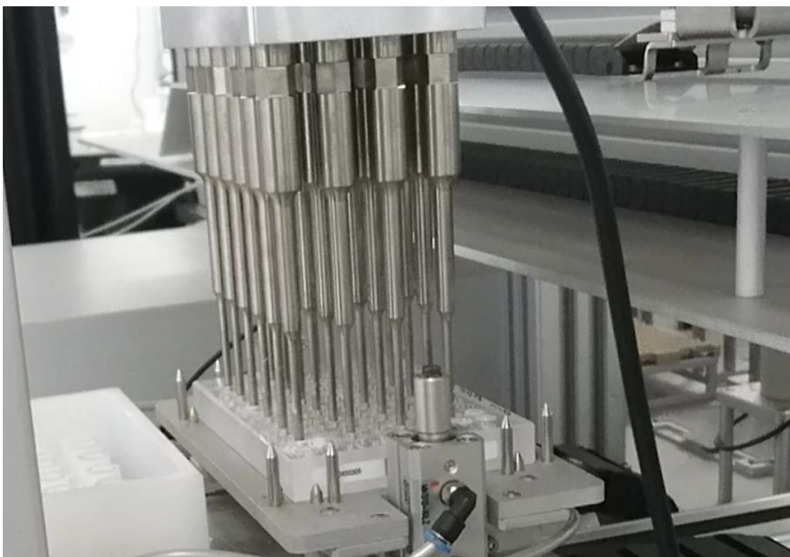
Figure 3.11 Photograph of sonication stage showing the 24-tip adapter in the wells of a quartz 96-well plate mid sonication.
