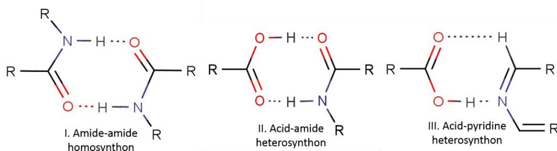
Figure 1.4 Examples of synthons. I. Amide-amide homosynthon, II. Acid-amide heterosynthon, III. Acid-pyridine heterosynthon.
