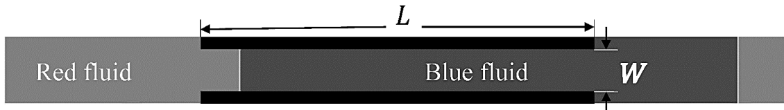
Figure 4. Geometry and initialization of the capillary filling problem. The portion in the center of the domain is a capillary tube of length L and width W . The red fluid is wetting with respect to the tube while the blue fluid is non-wetting.
