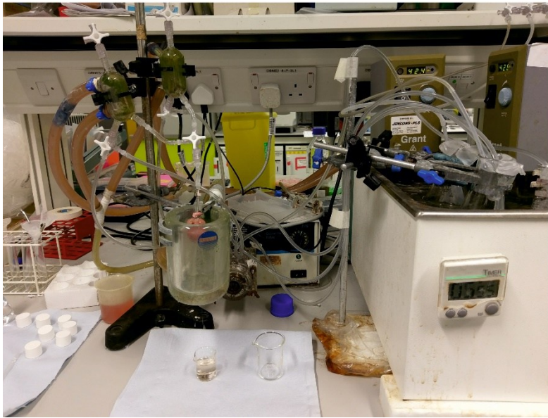
Figure 2-5. Langendorff perfusion system (A) and a cannulated heart (B).
