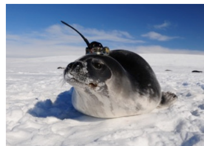
Figure 1 : Weddell seal carrying a CTD-SRDL instrument that collects temperature and salinity profiles while the animal is at sea (Credits: D. Costa).
