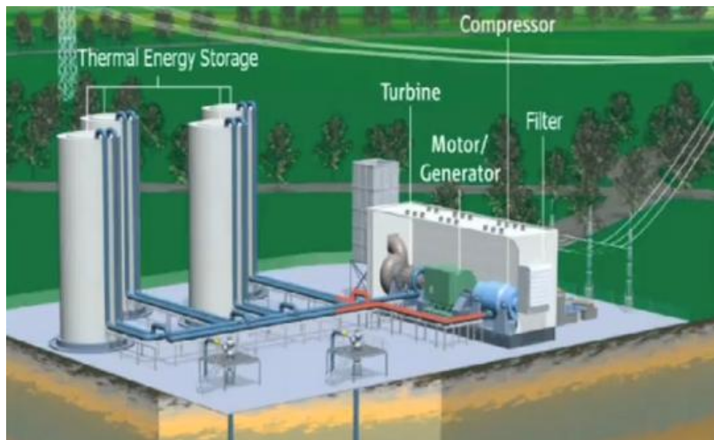
Figure 4-2 A-CAES with direct heat-exchange design [75]
