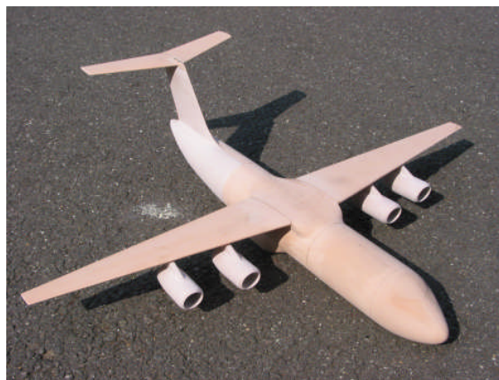
Figure 6 – Completed F-02 Wind Tunnel Model (Before Painting)
