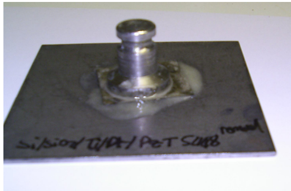
Figure 4-21 Test specimen ready for pull test
