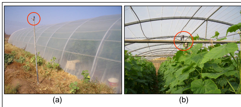
Fig. 4.6: The Delta-T photodiodes placed at 2 m height (a) outside and (b) inside Nizwa greenhouse
