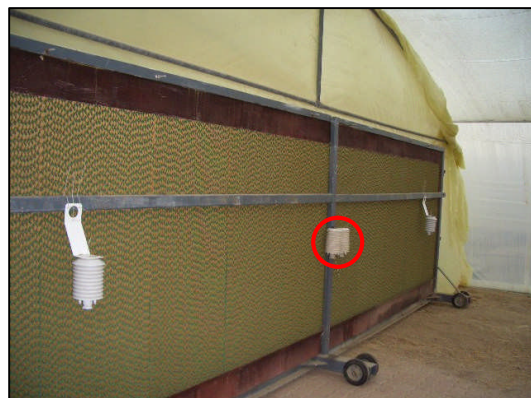
Fig. 3.4: The air washer used in the experiments and in this picture, the position of the shielded temperature/relative humidity sensor is enclosed by the circle
