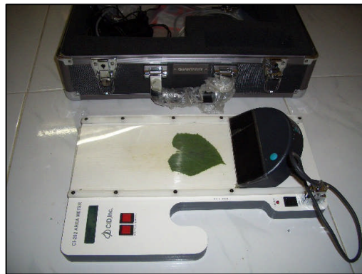
Fig. 4.7: The leaf area meter used to measure the area of cucumber leaves for the leaf area index estimation
