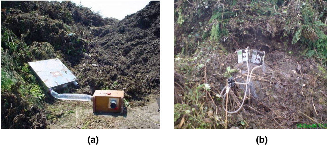
Figure 3.4- Bioaerosol sampling at Keenan Recycling incoming waste compost windrow (a) using the sampling hood (b) placing the sampling filters on the compost windrow.
