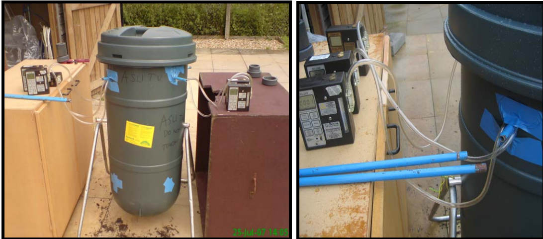
Figure 4.3-Images of the experimental chamber (Blackwall Aerobic Compost Tumbler) used for taking air samples for culture method and SEM analysis
