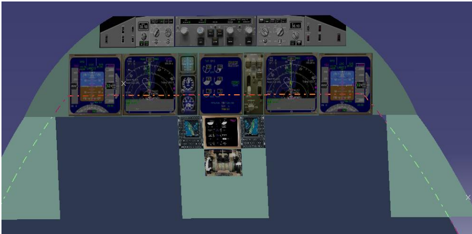
Appendix Figure B-1 Layout of cockpit in preliminary design
