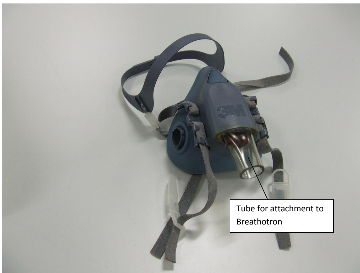
Figure 4 Particle mask (3M model no 750) adapted with tube for attachment to Breathotron
